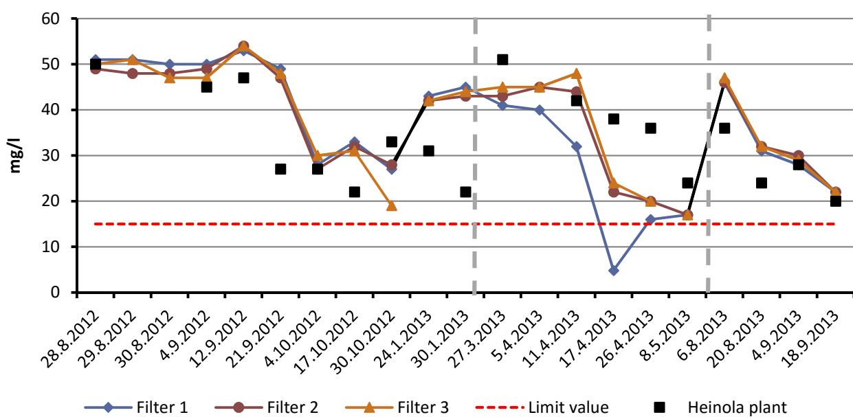
**Graph 4.** Ammonium nitrogen in filters **1**, **2** and **3** compared with the secondary settling output water at the Heinola waste water treatment plant. The vertical lines describe phases 1 – 3, due to maintenance.
